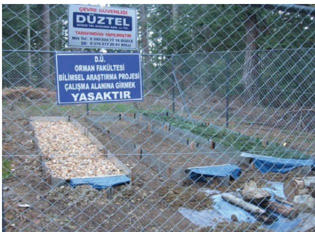
Figure 1. Establishment of runoff plots on skid trails Slika 1. Definiranje ploha otjecanja oborina na traktorskim vlakama
