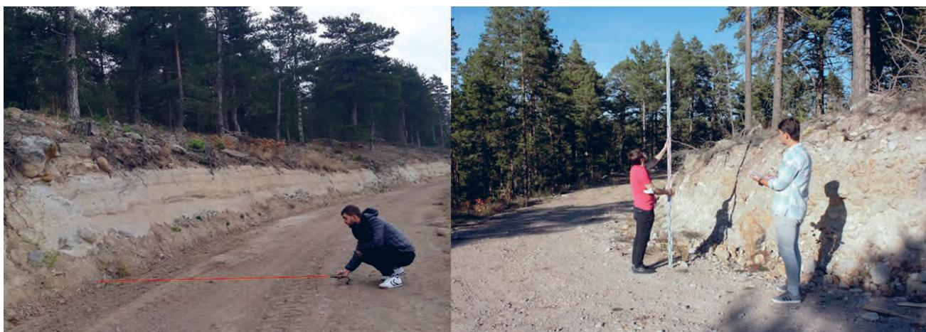
**Figure 8.** Measurement of cut slope width and height
