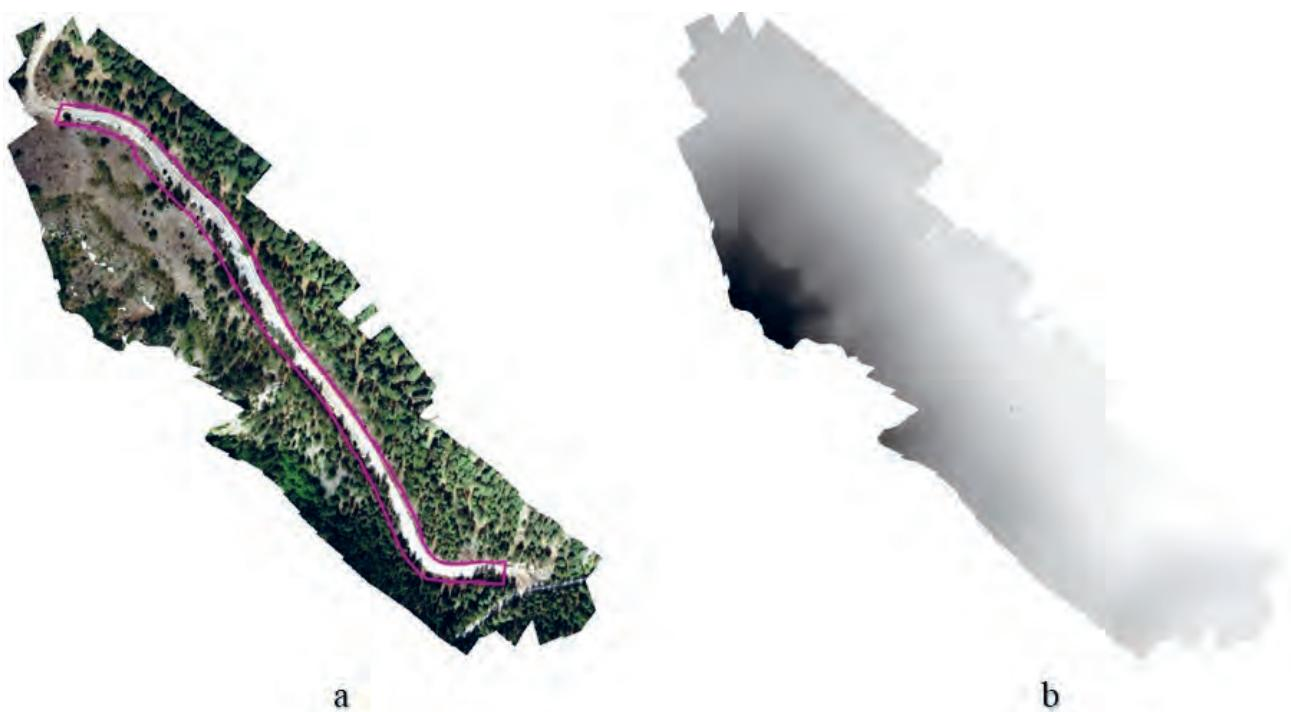
**Figure 13.** Orthophoto (a) and DEM data (b) of the study area after road construction
