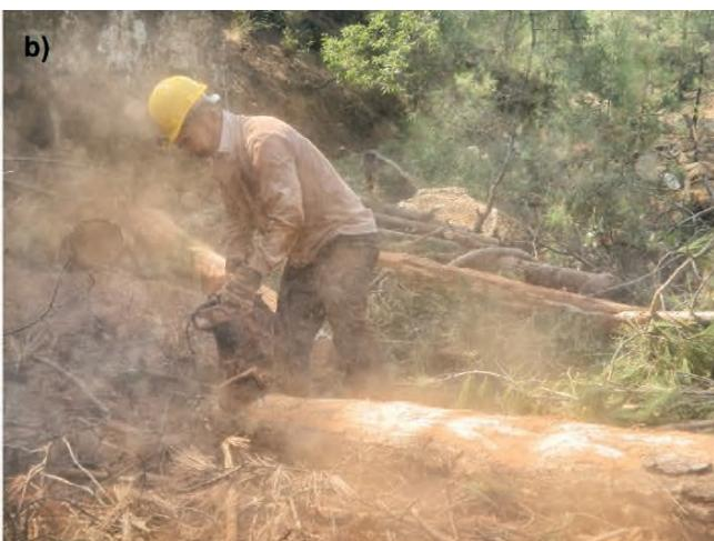
**Figure 3.** The moment of exposure to emitted exhaust gases from the chainsaw for an operator using low-standard work safety equipment (a: tree felling with chainsaw, b: debarking with chainsaw)
