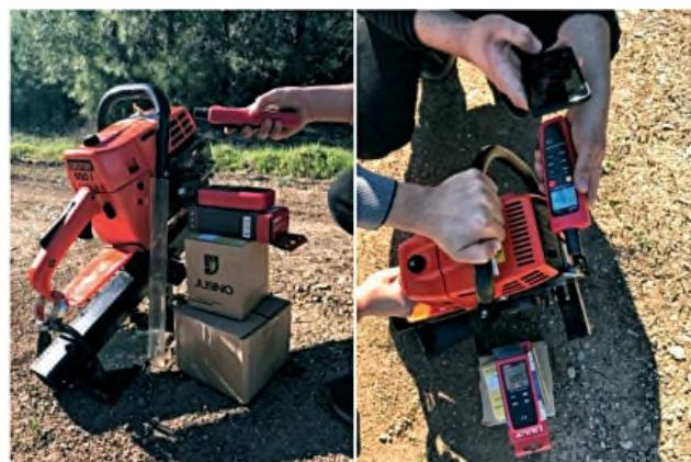
ring the measurement exceeds the exposure limit specified according to a short-term exposure limit (STEL) and a time-weighted average (TWA), the measurement tool will issue a luminous warning.
