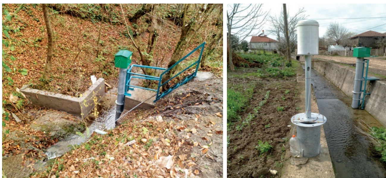
Figure 3. Streamflow gauging station installed in the FW (left) and the AW (right) Slika 3. Mjerna stanica vodotokova u FW (lijevo) i AW(desno)
