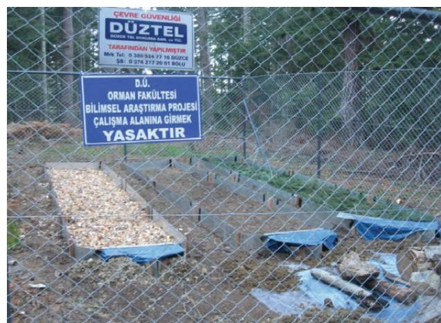
**Figure 1.** Establishment of runoff plots on skid trails
