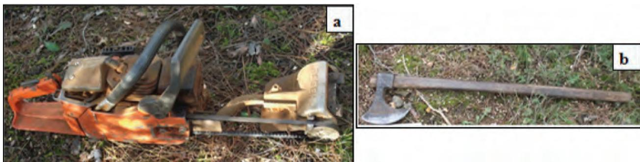
**Figure 2.** Chainsaw mounted debarking tool (a), and axe (b)
